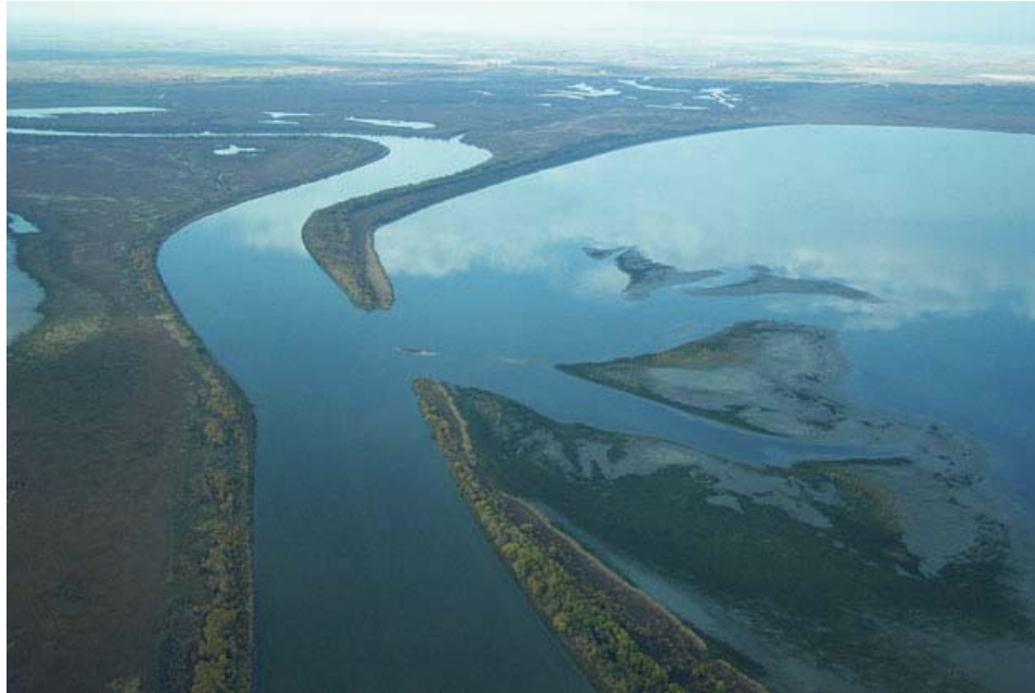
Fig. 5 The “Netley Cut” shown here was originally excavated from the Red River into Netley-Libau Marsh in 1913 but has eroded into a channel that now redirects from one-third to one-half of the entire river flow in the marsh (Photo credit: G. Goldsborough © Rights remain with the author)
